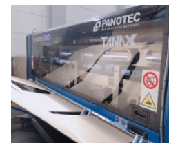
Introduced automatic packing material preparing machines capable of handling various types of product packing.
